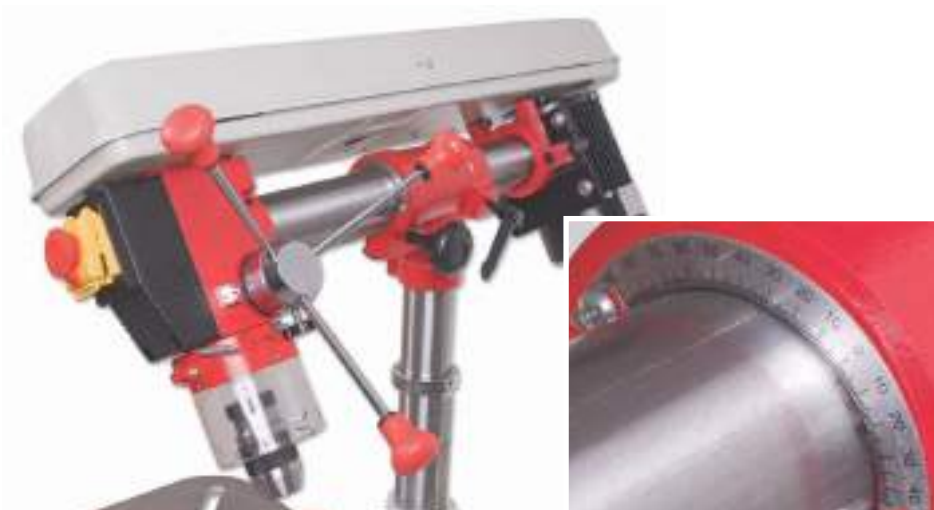
Loosen the horizontal column clamping handle (B). Pull out the vertical locking pin to un-lock the drill head column. Rotate + or - to the appropriate angle using the tilt pointer on the column then retighten the horizontal clamping handle to lock the head in position.
